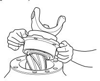
**Note:** Do not install cotter pin until carrier adjustments are completed.
