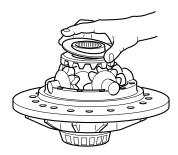
Align punch marks and install plain case half. Install capscrews and tighten to 114–140 lbs. ft. (155–190 N•m). Check differential for free rotation by turning side gear hub.
